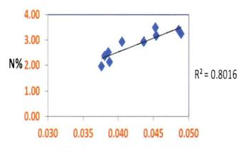
Fig. 3.7.1: Correlation between nitrogen content of cotton leaf and IR/LED value of N Guru
